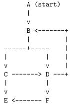
Let's represent the graph by a list of (x y z ...) where x can directly go to either y z .... (define \*graph\* '((A B)
